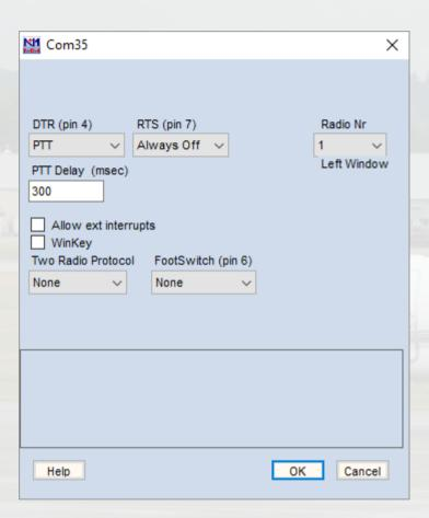
The **PTT Delay** value is set to work with a sequencer.
