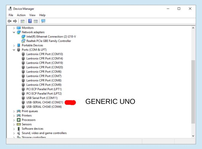
Download the IDE and Install it. That should also install the driver. If it doesn't, download and install drivers from http://www.wch.cn/download/CH341SER\_EXE.html
