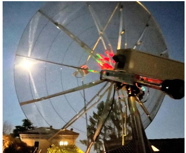
IQ2DB 3 m dish with Septum feed
