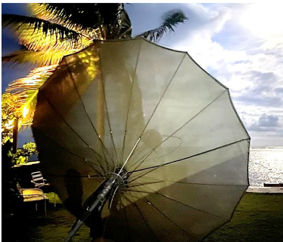
N1V's 2.4 m folding dish with circular patch feed in HI
