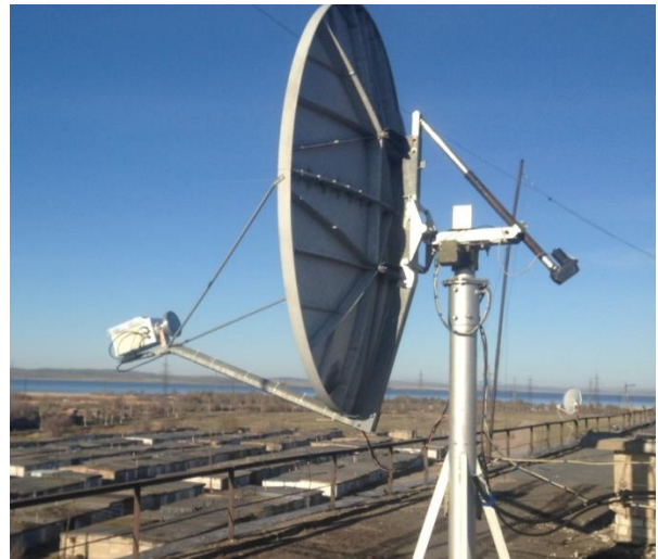
UN6PD's 1.6 m offset dish with 6 cm feed
