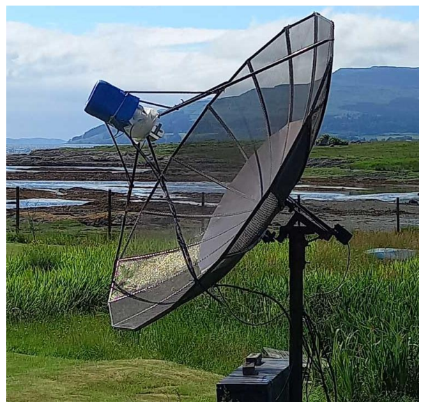
GM4PMK's 3.2 m dish used to put GM on 9 cm
