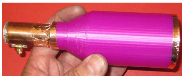
KN0WS 3 cm IMU horn made by 3D printing. Carl used copper tape to make inner part of horn conductive
