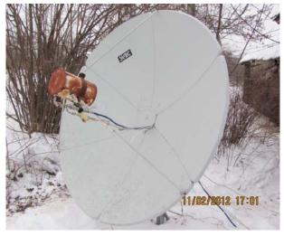
UA3TCF's 1.8 m dish used on 1296 with linear feed
