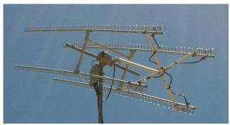
N6RMJ 4 loop yagi array for 23 cm
