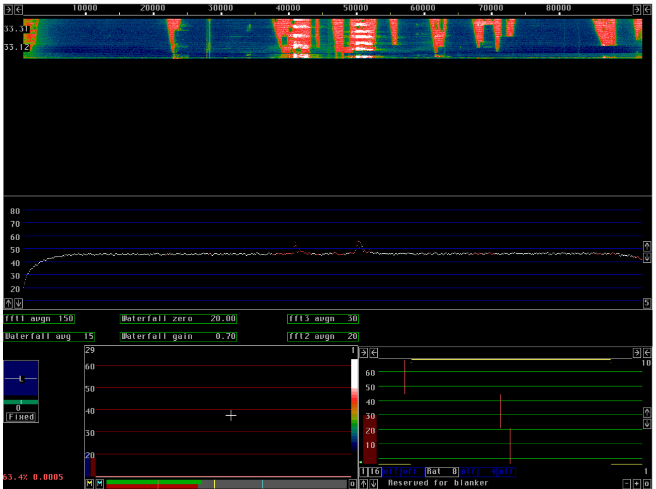
Fig 7. Smart and dumb blanker together. Dumb blanker threshold is very low and the red S/N control bar is low. Once a frequency is excluded it will stay excluded since the noise produced in excluded frequency bands by the dumb blanker is strong enough to keep them excluded. If patterns of this kind show up on the waterfall graph the red bar has to be moved upwards or the yellow line has to be moved more to the right. Increasing the waterfall averaging may also be helpful.
